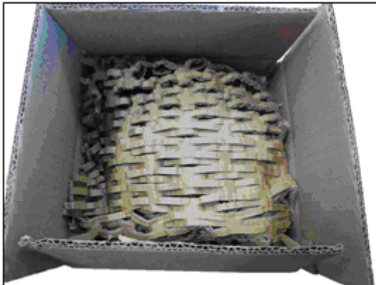
Example of acceptable cushioning material
